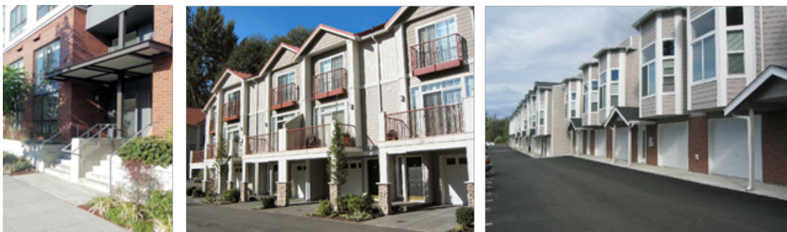
Figure 2. Good and bad examples of garage/entry configurations. The left example features a landscaped area and stoop to enhance the entry. The townhouses in the middle photo tuck the garages under the living units to reduce their visibility (note that this is a private roadway). In the right image, the lack of landscaping is a glaring omission, and is not acceptable.
