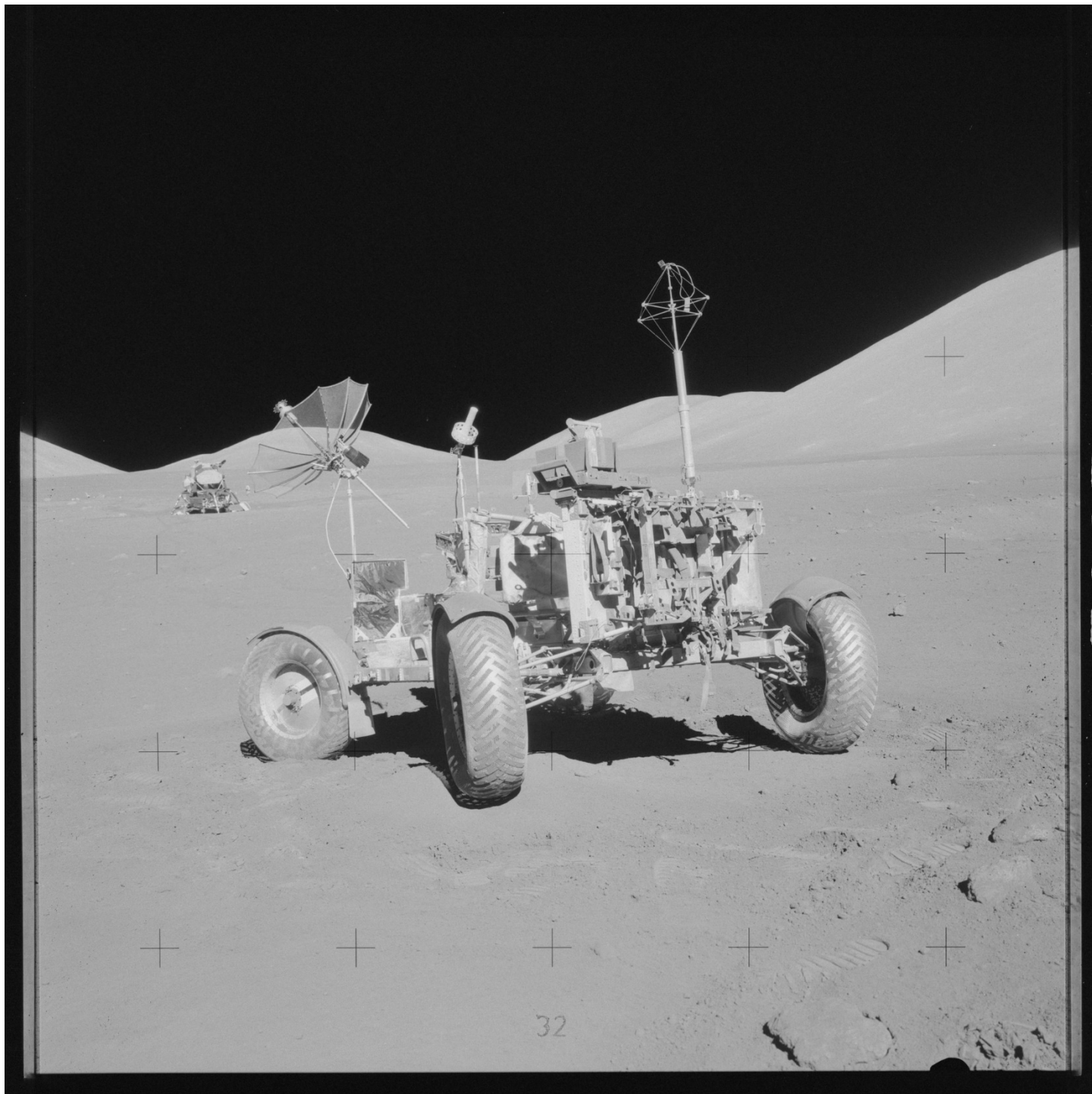
Figure 23: Apollo 17 – the LRV is shown in its final parking spot, with the LM in the background. By the time Eugene Cernan took this photograph, he had already removed the replacement fender at the right rear and, also, had removed the left rear fender extension. NASA photograph AS17-143-21931, taken Dec. 13, 1972. Digital image archived by NASA at: https://www.flickr.com/photos/projectapolloarchive/21036715824
